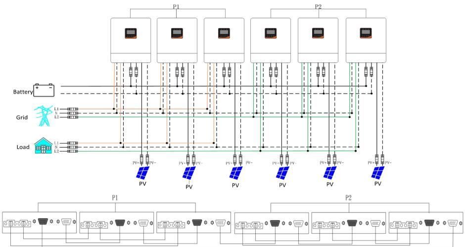
**f) Seven hybrid inverters of the system connected in two phase:
