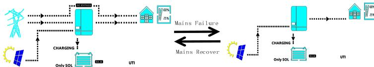
3) **Inverter First:** switch to Mains Power supply only when the battery is under-voltage. This mode uses DC energy to the maximum extent and is used in regions with stable power grid.
