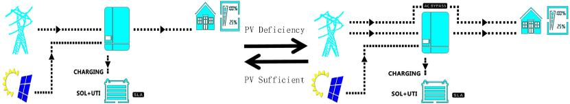
4) **Only Solar:** Only PV charging, no mains charging is initiated. This is the most energy-efficient mode and the battery power comes from solar energy, which is usually used in regions with good daylighting conditions.
