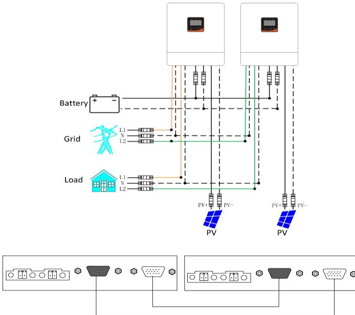
**b) Three hybrid inverters of the system connected in two phase:
