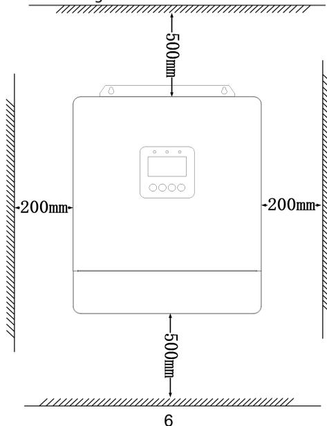
**⚠ Warning: Danger of explosion! Never install the hybrid inverter and lead-acid battery in the same confined space! Also do not install in a confined place where battery gas may collect.**
