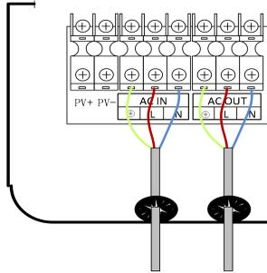
5) Make sure the wires are securely connected.
