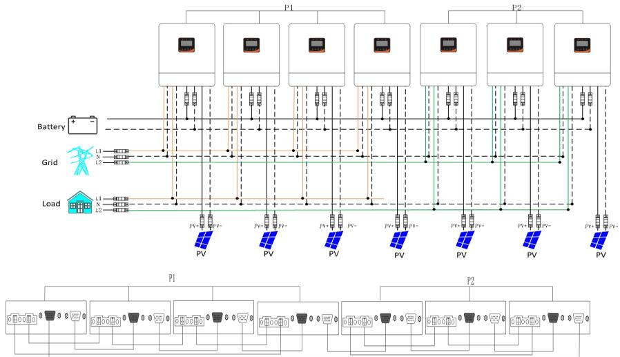
**g) eight hybrid inverters of the system connected in two phase:**
