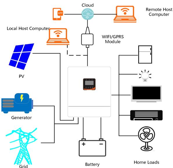
GST48 series is a new hybrid solar charge inverter, which integrates solar energy storage & means charging energy storage and AC sine wave output. It adopts DSP control and advanced control algorithm, it has high response speed, high reliability and high industrial standard. Four charging modes are optional, i.e. Only Solar, Mains Priority, Solar Priority and Mains & Solar hybrid charging; and two output modes are available, i.e. Inverter and Mains, to meet different application requirements.
