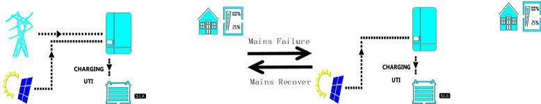
3) **Hybrid Charging:** hybrid charging of PV and Mains Power, give priority to PV MPPT charging, and supplement Mains Power when PV energy is insufficient. When the PV energy is sufficient, the Mains Power will stop charging. This is the mode of fast charging and suitable for unstable areas of power grid, and can provide sufficient backup power at any time.
