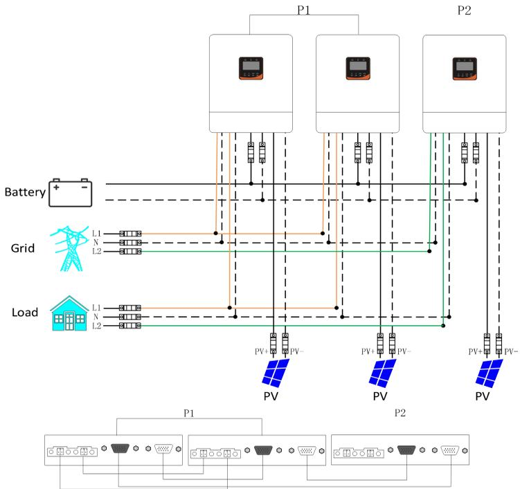
**c) Four hybrid inverters of the system connected in two phase:
