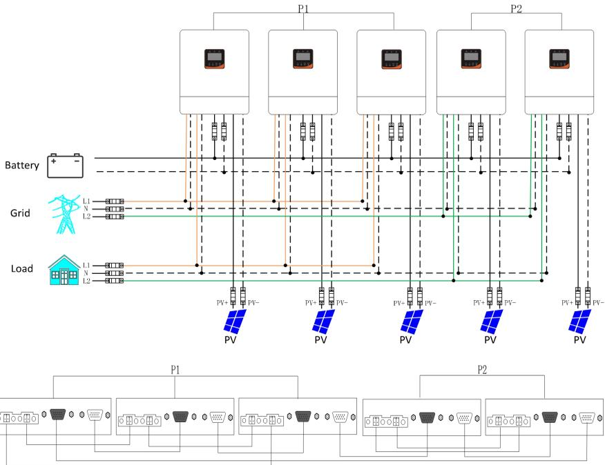
**e) Six hybrid inverters of the system connected in two phase:**
