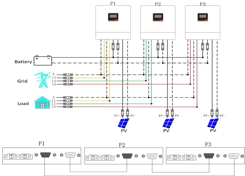
**b) Four hybrid inverters of the system connected in three phase:
