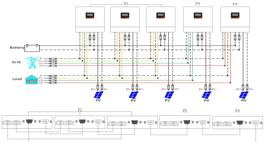
**d) Six hybrid inverters of the system connected in three phase:**
