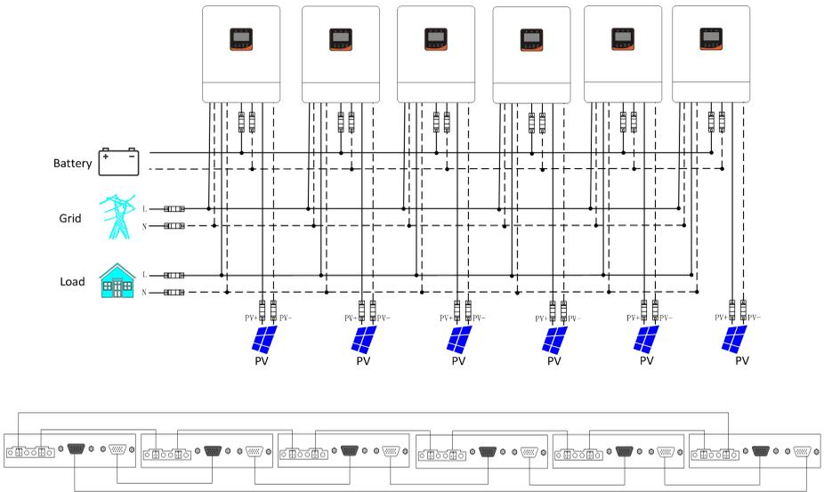
**f) Seven hybrid inverters of the system connected in parallel:**
