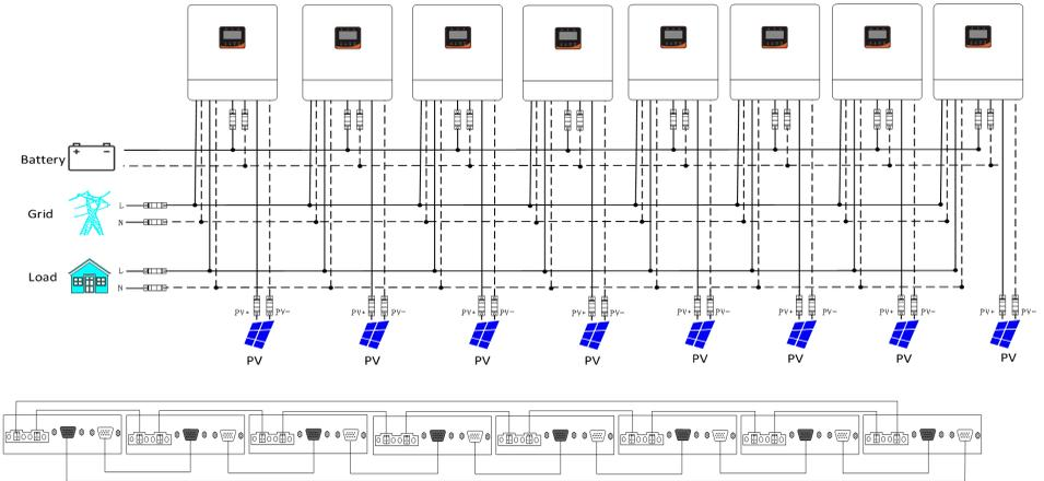
**h) Nine hybrid inverters of the system connected in parallel:**
