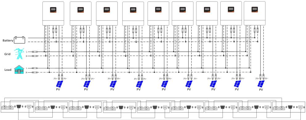
**5.4 Schematic diagram of parallel connection in split phase**
