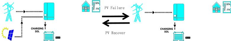
2) **Mains first:** priority shall be given to charging by Mains Power, and charging with PV power will be started only when the Mains has failed.
