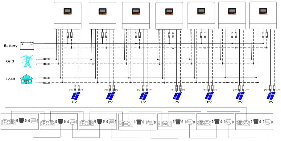
**g) Eight hybrid inverters of the system connected in parallel:**
