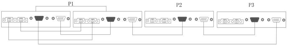
**c) Five hybrid inverters of the system connected in three phase:
