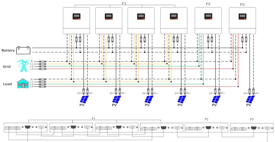
**e) seven hybrid inverters of the system connected in three phase**
