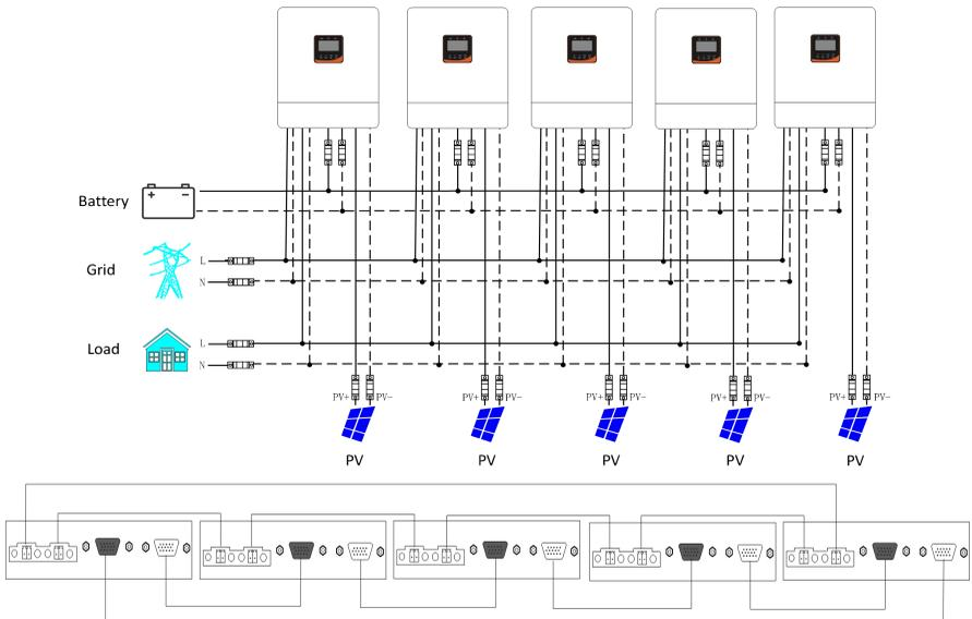
**e) Six hybrid inverters of the system connected in parallel:**
