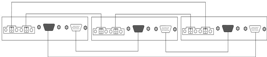
**c) Four hybrid inverters of the system connected in parallel:**
